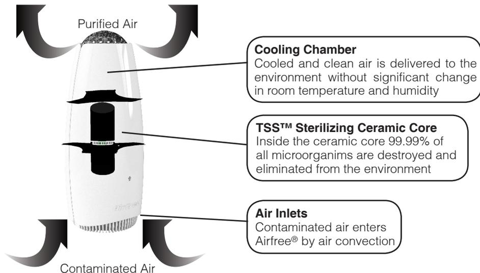
Regardless of how hazardous a virus, fungus or bacteria might be they are fully destroyed by the powerful heat inside the TSS™ ceramic core mini ducts. The heat inside the ceramic core forces sterilized air up to the heat exchanger causing air convection, which generates negative pressure underneath the ceramic core, so contaminated air is “sucked” in at Airfree® bottom air inlets in a continuous, silent, and efficient air flow.
